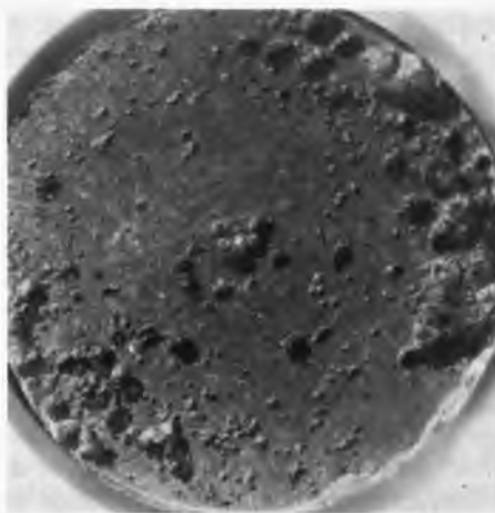
Fig. 18. Attack mechanism on a Cr steel in fast-flowing media containing H_2S . First phase (left): formation of pits; second phase (right): spreading of the pits and crumbling of entire surface areas (magnification about 10x).
