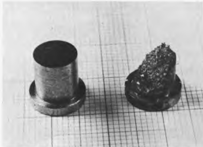
Fig. 11. Significance of the critical flow velocity for erosion corrosion on stainless steels in media containing chloride (left: critical flow velocity not exceeded; right: critical velocity exceeded). Test duration 200 h in both cases.
