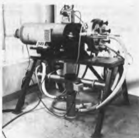
Fig. 5. High-velocity testing machine (left: dc motor; right: casing with disk-shaped impeller).
