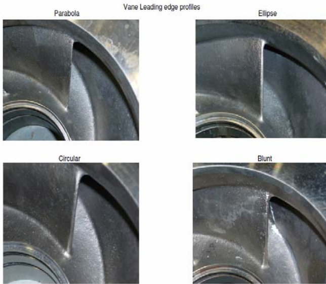
Figure 5: Cast Impellers with different leading edge profiles
