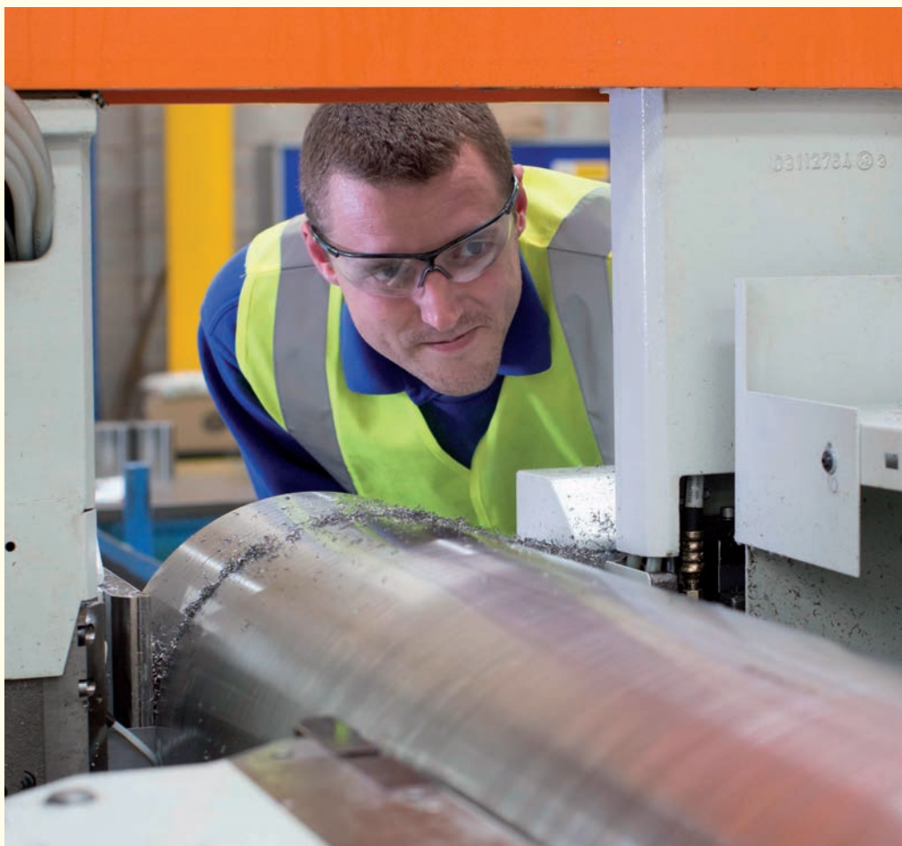
Large diameter stock being cut by Langley Alloys on one of the KASTOtec bandsaws
